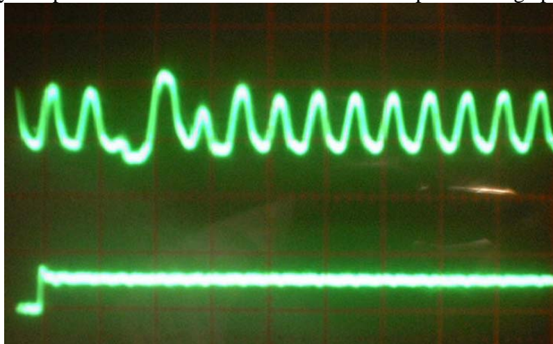
Figure 1. Waveform of the unsynchronized VMSK/2b Single Sideband ahead of narrow bandpass filtering. The early / late transitions of the VMSK modulation are seen as abrupt phase changes lasting 2-3 cycles. The remainder of the time, the signal is almost constant in frequency and phase. The modulation is in the form of phase change pulses.
