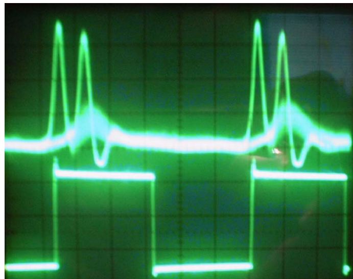
Fig. 3. Encoding and SSB modulation produce phase modulation pulses.
