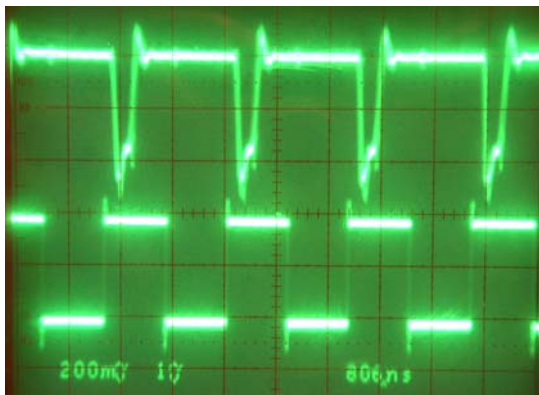
Figure 6, Recovered information spikes with no modulation deviation. Taken from the IF detector output after multiple stages of UNB zero group delay filtering. The spikes in Figure 6 are demodulated with the frequency to voltage
