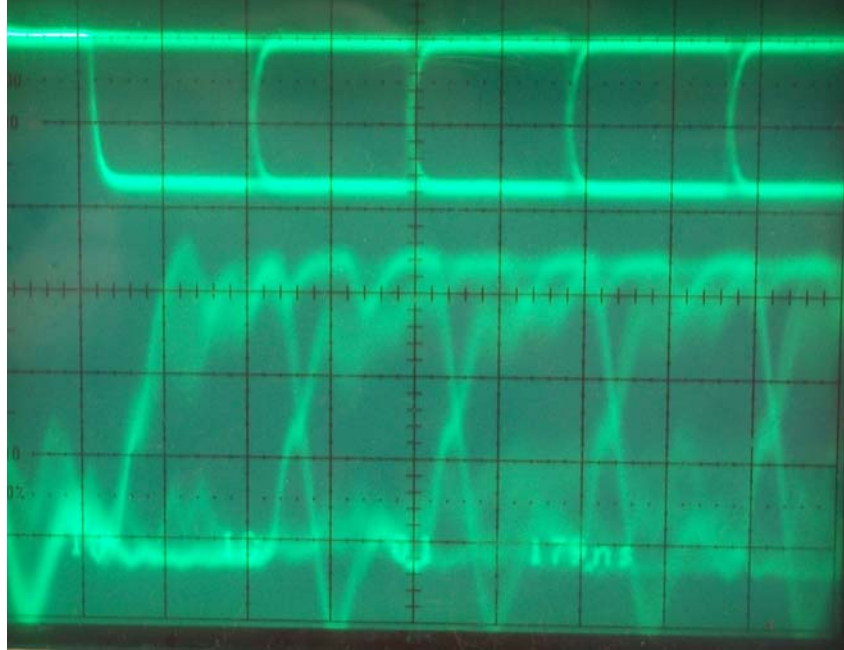
Figure 11. The EYE pattern after the filter. The scale is 1 Volt per division. There is a slight increase in output voltage level indication no phase loss. The rise and fall slope is slightly longer in time. The spectrum is that shown in figure 8 where the filter peak is to the left of the signal and approximately 4-5 dB higher. This indicates a reference phase approximately 60 degrees off signal average, similar to that seen in Figure 6.
