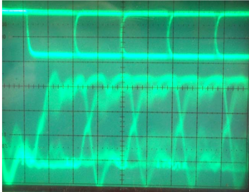
Figure 11. The EYE pattern after the filter. The scale is 1 Volt per division. There is a slight increase in output voltage level indicating no phase loss. The rise and fall slope is slightly longer in time. The spectrum is that shown in figure 8 where the filter peak is to the left of the signal and approximately 4-5 dB higher. This indicates a reference phase approximately 60 degrees off signal average, similar to that seen in Figure 6.
