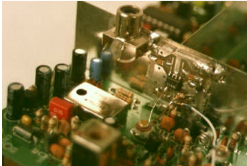
Fig.10. 24 MHz injection jack and 455MHz to 431MHz mixer on Hamtronics T304 Exciter. The 8 pin mixer is Avantek IAM81008.
