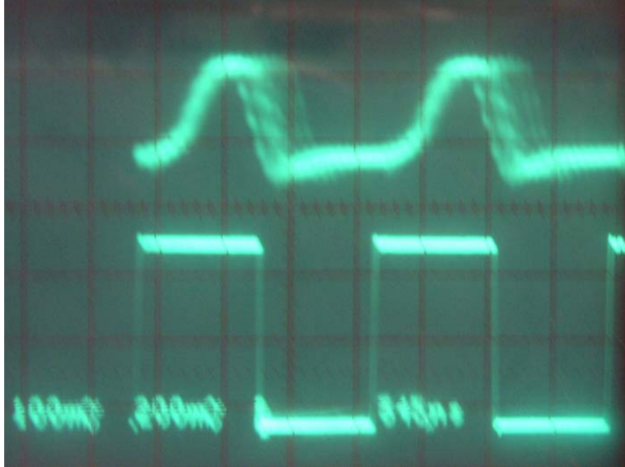
Figure 5. Detected output of 2 stages of TRS filter. The phase loss is from 120 to 40 degrees. Detector circuit RC rise time using Fig. 2 limits the minimum number of altered cycles that can be used. This is not an optimum detector, but it allows measurement of the phase loss in the filters from the amplitude of the detected signal from before and after the filter.
